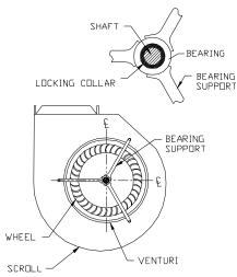
FIGURE 4 - CONCENTRIC WHEEL ALIGNMENT
